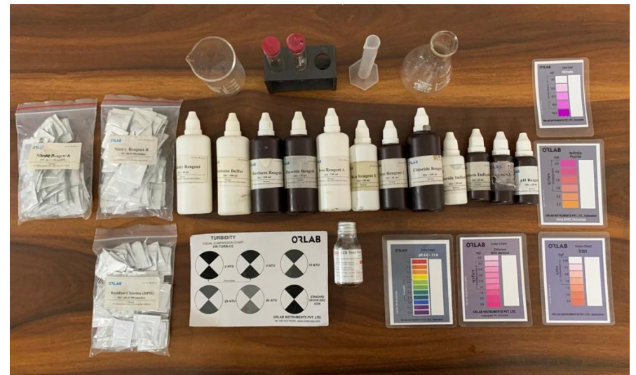
Components of the water testing kit
